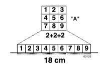
In this way it is easy to understand how it is possible for a droplet, which is turned into smaller ones, to double up, triple or quadruple its coverage capacity. It is also easily understood, if one can count on a certain quantity of water, how the possibilities for coverage can be different and are strictly linked to the method used to make spray droplets.
