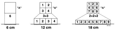
In this way it is easy to understand how it is possible for a droplet, which is turned into smaller ones, to double up, triple or quadruple its coverage capacity. It is also easily understood, if one can count on a certain quantity of water, how the possibilities for coverage can be different and are strictly linked to the method used to make spray droplets.
