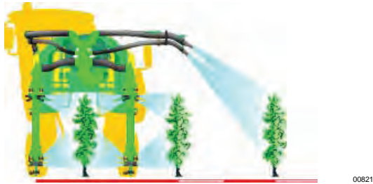
TC.8M4C - Cover 3 rows - distance between the rows 2,00 ÷ 2,60 meters
