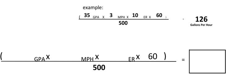
5. SPRAYHEAD CHART Find the GPH below which most closely matched the number you determined in the formula on the opposite page. Set the pressure gauge and the yellow metering dics accordingly
